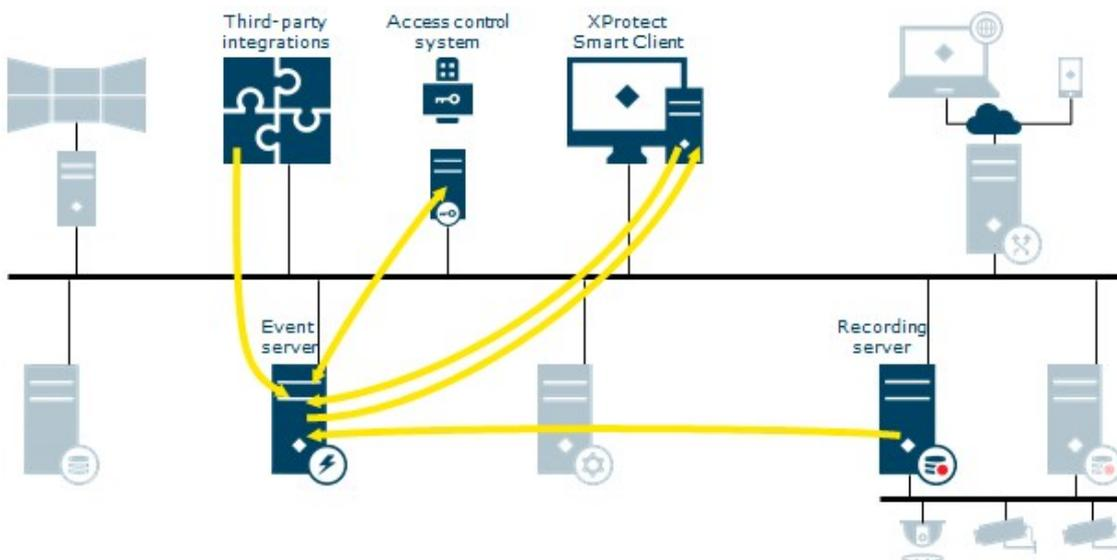
The event server sends data to XProtect Smart Client to show in alarm list, XProtect Access or the map overview. The event server Plug-in is a client to the access control system. The XProtect Smart Client user responds to the notification and returns data to event server.
