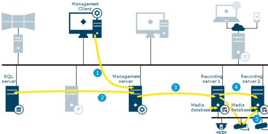
1. The user moves hardware from recording server 1 to recording server 2 in Management Client
