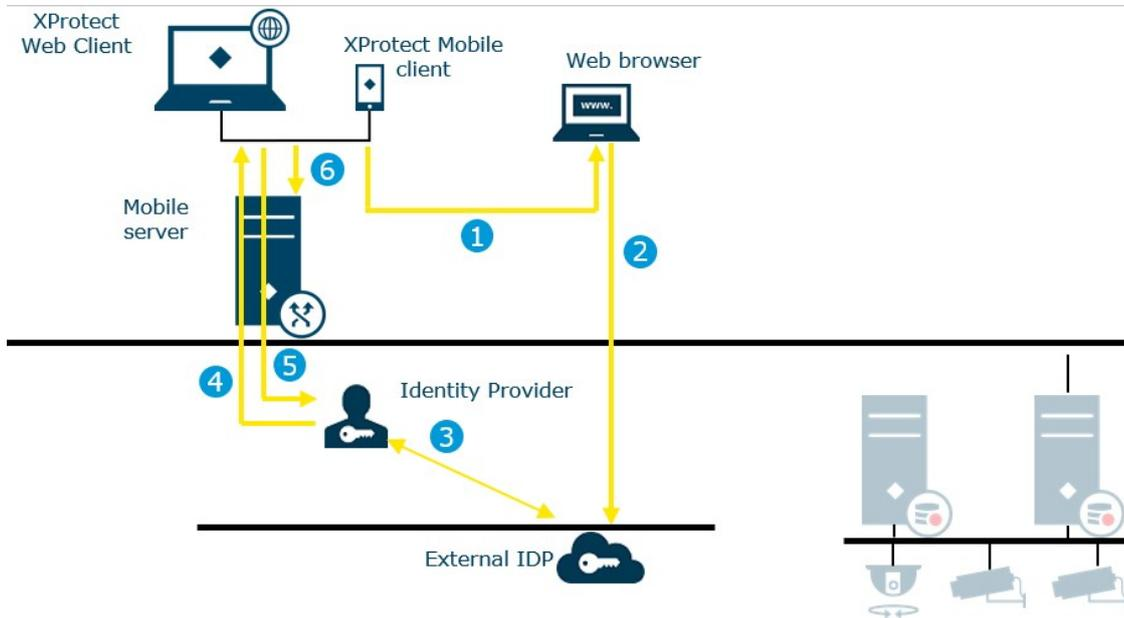
1. In XProtect Web Client or in the XProtect Mobile client, the user selects to log in via an external IDP. The login request launches a web browser.
