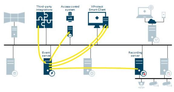
The event server sends data to XProtect Smart Client to show in alarm list, XProtect Access or the map overview. The event server Plug-in is a client to the access control system.
