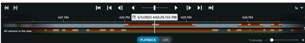
The main timeline displays an overview of time periods with recordings from cameras and other devices in your current view. The main timeline is available on the views tabs and has various controls you can use to navigate your recordings during investigations or to select recording sequences for export, protection with evidence locks, addition of bookmarks, or other.
