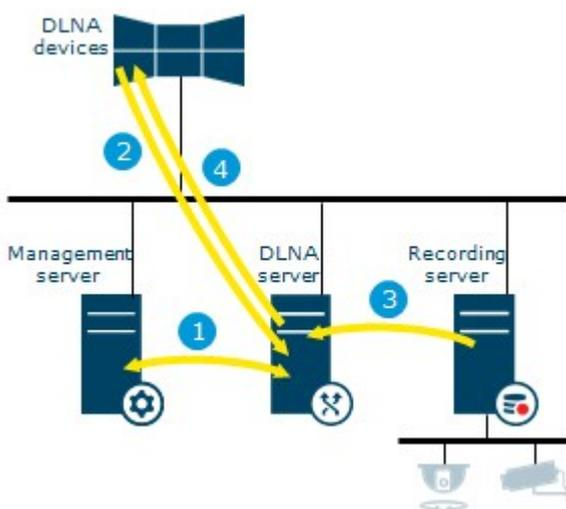
1. During start up of the XProtect DLNA Server service, the XProtect DLNA Server connects to the management server to authorize itself with the provided credentials. After authorization, the XProtect DLNA Server starts and is ready to send H.264 video streams from the cameras to the DLNA devices.
