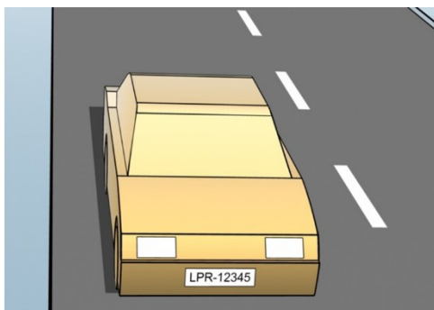
Distance to the car; to define the area where LPR analyzes license plates
