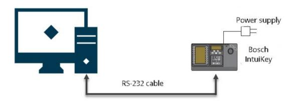
This connection requires a standard Null modem RS-232 cable. Connect one end of the RS-232 interface cable to the 9-pin RS-232 Serial Port located on the far right side of the rear of the Bosch IntuiKey Keyboard. Connect the other end of the RS-232 interface cable to a COM port on the PC.
