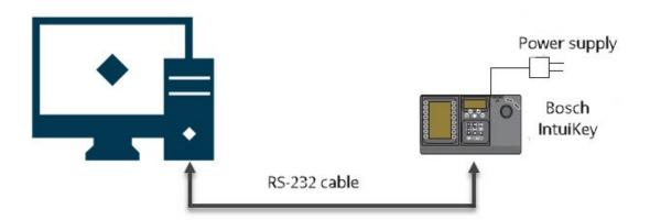
This connection requires a standard Null modem RS-232 cable. Connect one end of the RS-232 interface cable to the 9-pin RS-232 Serial Port located on the far right side of the rear of the Bosch IntuiKey Keyboard. Connect the other end of the RS-232 interface cable to a COM port on the PC.
