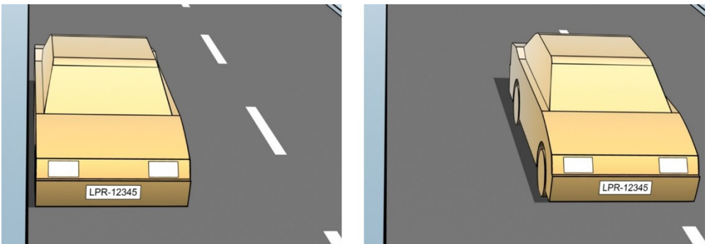
Distance to the car to define the area where LPR analyzes license plates
