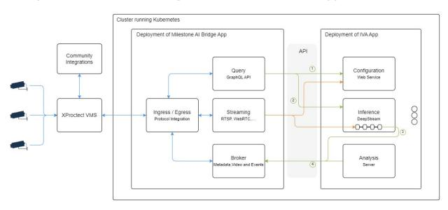
This is one example of a simple deployment of the Milestone AI Bridge in connection with the XProtect VMS and an Intelligent Video Analysis (IVA) application.
